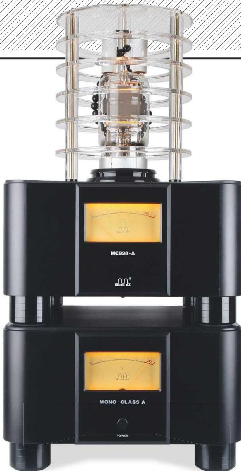
**LEFT:** Looking more like a contraption from a steampunk novel than a piece of domestic hi-fi, this sturdy two-box (mono) amplifier is well finished and crowned by its striking FU80 tube
